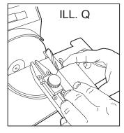
To grind the secondary relief and clearance angles, adjust the desired angle on the table's side protractor and set the stop pin forward a small amount and grind one flute. Check frequently to see how much material is being removed. If not enough and you are against the stop pin, move the pin inward. If you have removed enough and you are not against the pin, hold the tool against "stopped" wheel and reset pin stop. After establishing pin placement, do the other flutes.
