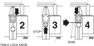
Double check that block is flat against tool stop and the "Stop Pin" is ahead of the block. Center tool with diamond wheel edge and LOCK table in position.
