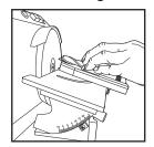
Set desired face angle on the table's side protractor. Place Collet Block against right side of tool stop. Holding it tight against the tool stop, move table until the
